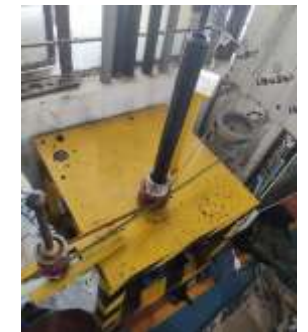
Cop Vibration Checking Arrangement
